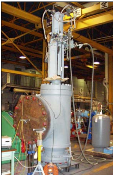
Figure 1: 30" Propane Compressor Antisurge Valve
