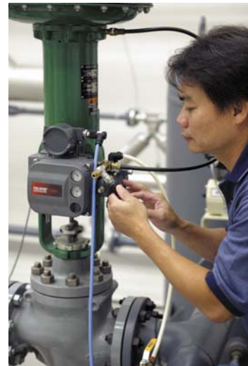
PlantWeb™ Performance Lab components include FIELDVUE® DVC instruments and AMS ValveLink® software with Performance Diagnostic (PD) capabilities.
